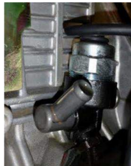
Injector pump inlet
