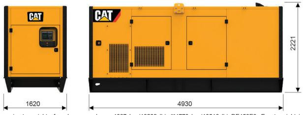
Approximate weight of enclosure package: 4667 kg (10289 lb), \*\*4770 kg (10516 lb) DE450E3. Exact weight is dependent on options. Enclosure weight includes: Sound attenuated enclosure, exhaust system, base and generator set.
